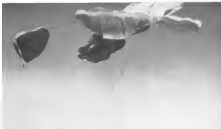
ARMY self-powered gas starts to swing on parachute slings. Last five feet of platform will extend around vehicle (top left). Gun falls in Junk under its 130 ft. dia. canopy which help to stop oscillation. Note distribution bags under platform (upper right). Automatic device cuts canopy loose on landing (below).
